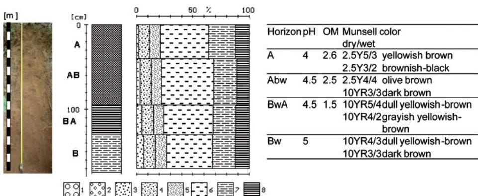
Fig. 4. Properties of soil profile CH2. Grain size composition: 1 – coarse gravel ( $> 16$  mm), 2 – fine gravel (2–16 mm), 3 – coarse sand (0.5–2.0 mm), 4 – medium sand (0.25–0.50 mm), 5 – fine sand (0.063–0.25 mm), 6 – coarse silt (0.02–0.063), 7 – fine silt (0.004–0.02 mm), 8 – clay (< 0.004 mm)
