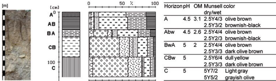
Fig. 8. Properties of soil profile GB1 (Grain size composition see Fig. 4)
