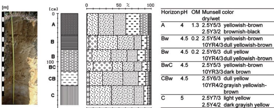
Fig. 7. Properties of soil profile RC1 (Grain size composition see Fig. 4)
